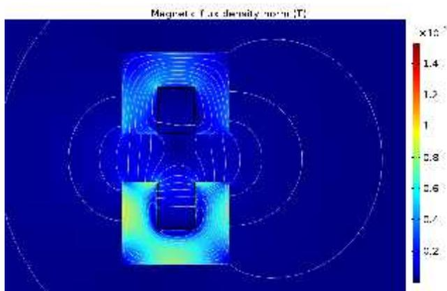
Figure 8. Magnetic flux density on amorphous core with 7 mm air gap when the air gap is equal to 3.5 mm.
