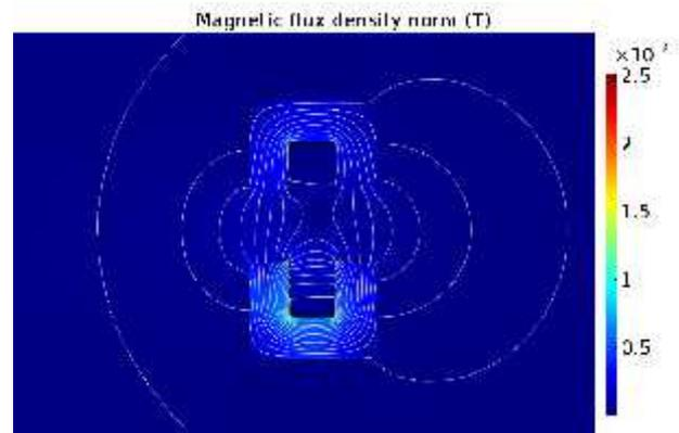
Figure 9. Magnetic flux density on ferrite core with 10 A load when the air gap is equal to 3.5 mm.
