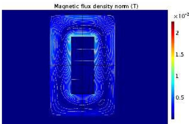
Figure 7. Magnetic flux inside amorphous core when there is no air gap between Tx and Rx. A 10 A load is connected to Rx.
