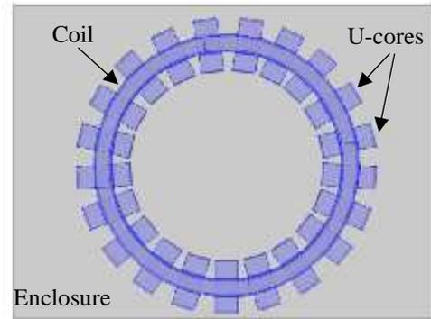
Figure 5. Top view of transformer with coil and U-cores are highlighted in blue.
