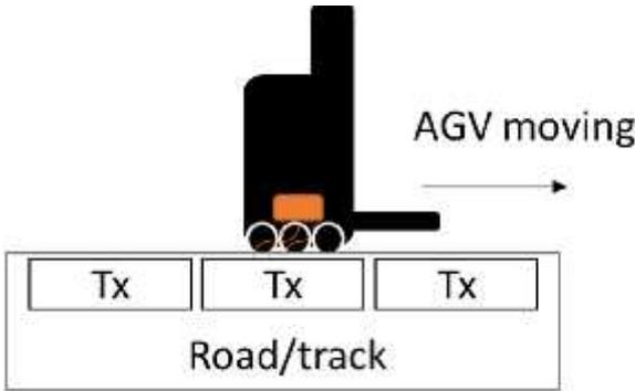
Figure 3. Dynamic WCS transferring energy to a moving electric vehicle.
