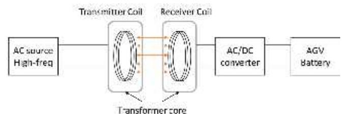
Figure 2. Diagram of WPT that has ferromagnetic cores on each end.
