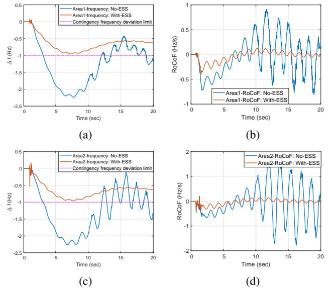
Fig. 7: Variations in frequency and RoCoF when fault applied in area-2 (a) frequency of area-1; (b) RoCoF of area-1; (c) frequency of area-2; (d) RoCoF of area-2.
