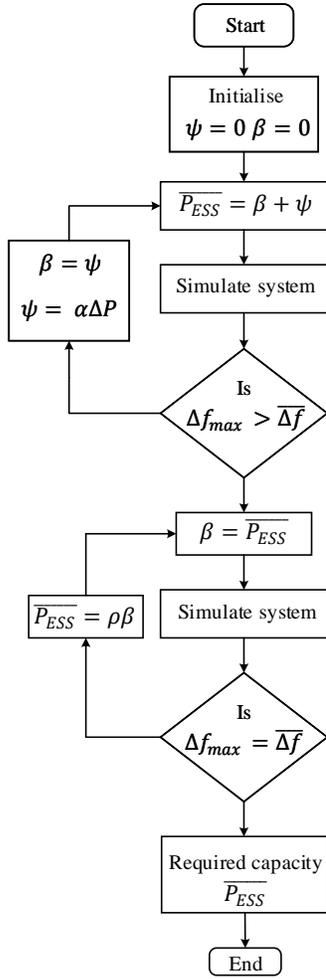
Fig. 2: Flowchart of capacity estimation algorithm.
