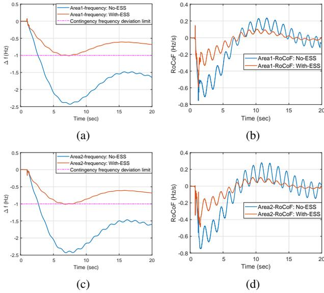
Fig. 5: Variations in frequency and RoCoF when fault applied in area-1 (a) frequency of area-1; (b) RoCoF of area-1; (c) frequency of area-2; (d) RoCoF of area-2.
