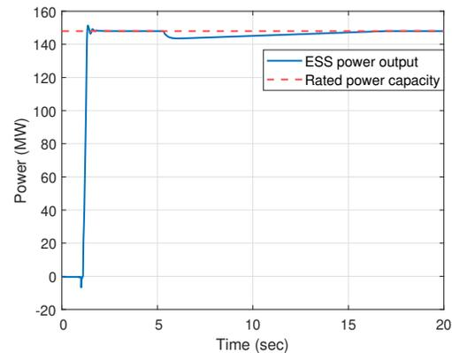
Fig. 8: Power output of ESS when fault applied in area-2.
