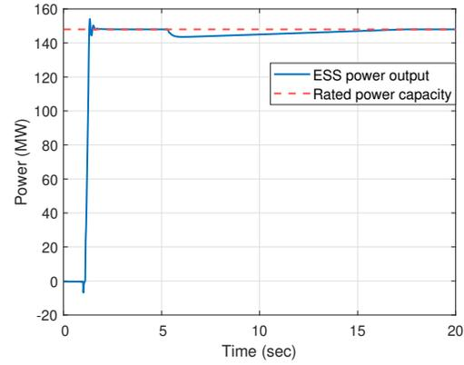
Fig. 6: Power output of ESS when fault applied in area-1.
