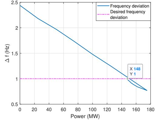
Fig. 4: Variation in power capacity of energy storage with the frequency nadir.
