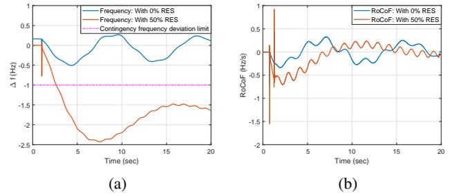
Fig. 3: Variations in (a) system frequency; (b) RoCoF.
