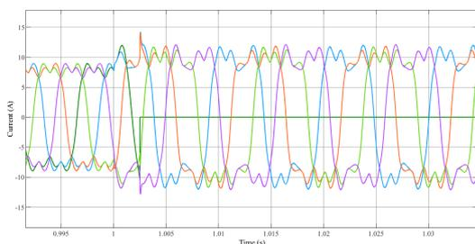
Fig. 7. Optimised current reference waveforms during fault occurrence
