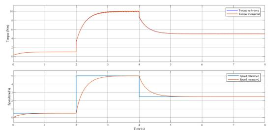
Fig. 9. Torque and speed waveforms in healthy conditions
