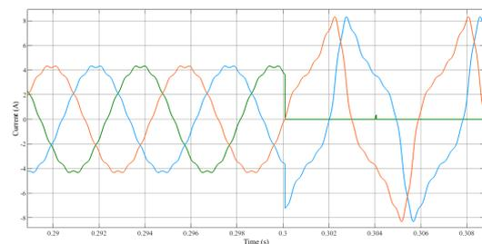
Fig. 4. Fault compensation current waveforms during fault occurrence
