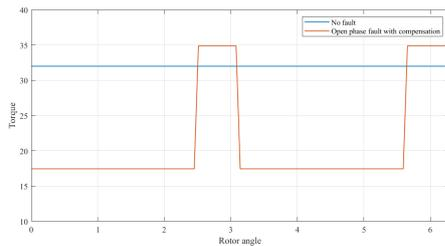
Fig. 1. Torque production before and after single open-phase fault in [7]
