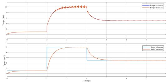
Fig. 10. Torque and speed waveforms with open phase fault
