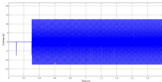
Fig. 6. Neutral line current before and after fault
