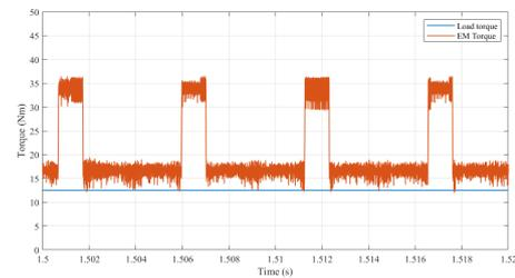
Fig. 3. Torque production after single open-phase fault with current correction
