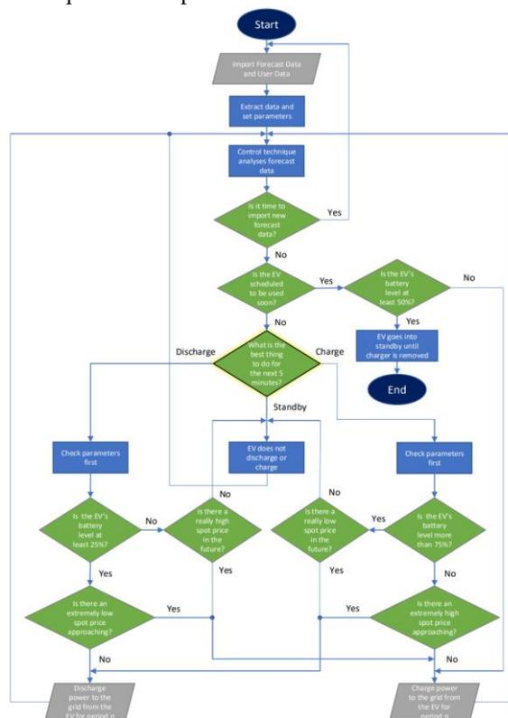
Fig. 2. Logic flowchart of the proposed advanced control technique.
