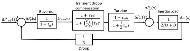
Fig. 3: Block diagram of a hydro power generator
