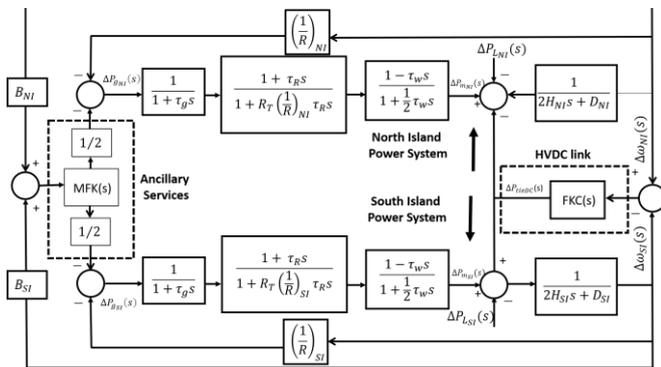
Fig. 6: Two-area LFC model of New Zealand power system
