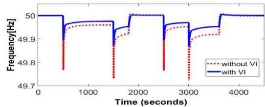
Fig.10: Frequency response in North Island (low inertia condition) – with and without virtual inertia
