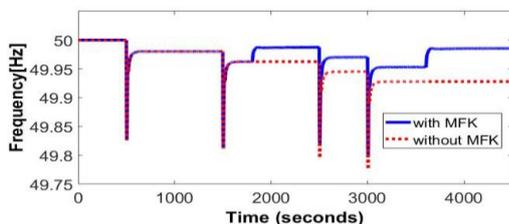
Fig. 9: Frequency response in South Island – with and without MFK
