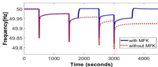
Fig. 8: Frequency response in North Island – with and without MFK
