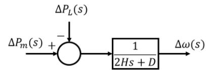
Fig. 1: Generator and load block diagram [13]
