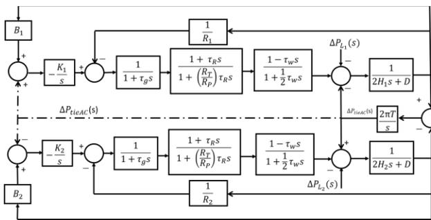
Fig. 4: AGC of a two-area control system
