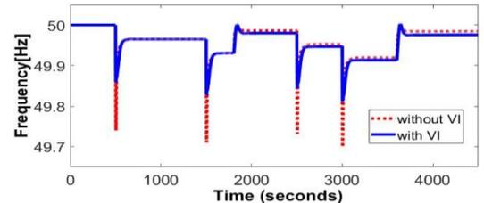
Fig. 11: Frequency response in South Island (low inertia condition) – with and without virtual inertia
