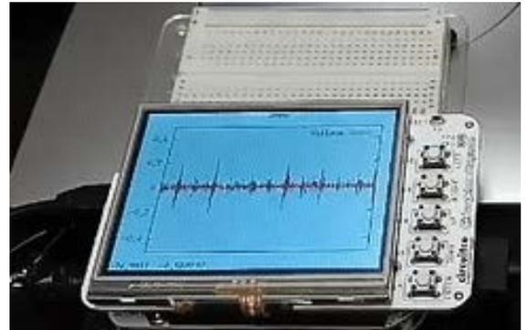
Fig. 7. Implementation of an LCD cape to plot the classified signals.
