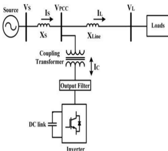
Fig. 5. Basic configuration of D-STATCOM [6]
