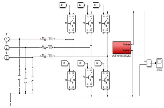
Fig. 6. Modelling of D-STATCOM in MATLAB
