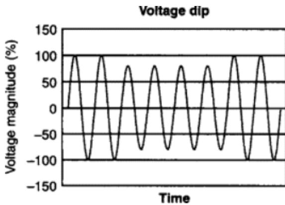
Fig. 2. Voltage sag/dip [5]
