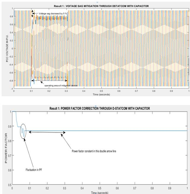
Fig. 11. Simulation Waveform of voltage profile & power factor with D-STATCOM
