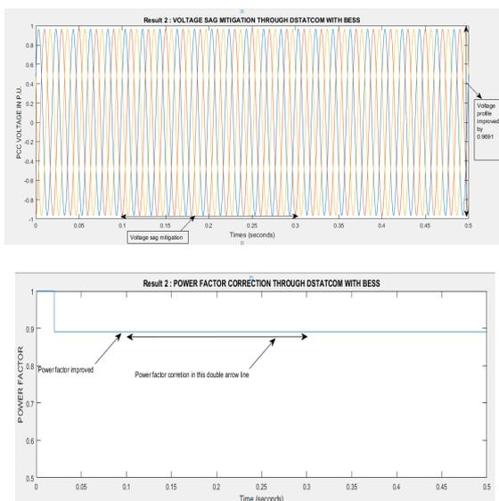
Fig. 12. Simulation Waveform of voltage profile & power factor with D-STATCOM+BESS
