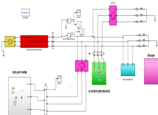
Fig. 8. Simulation Model
