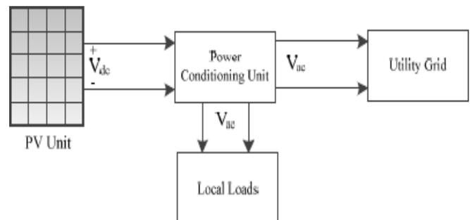
Fig.1. Grid connected Solar PV system [3]
