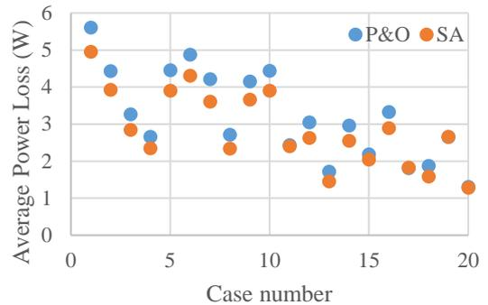
Fig. 3 Average power losses in the diode for each case with the two MPPT methods
