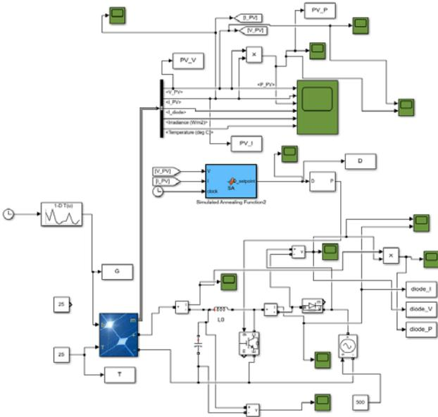
Fig. 2 Simulation model with the SA-based MPPT method
