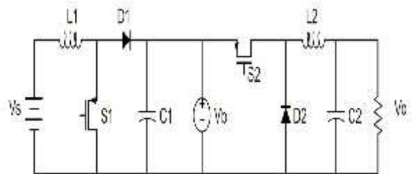
Figure 3: Conventional Boost Buck Converter
