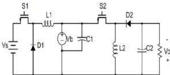
Figure 5: Conventional Buck into Buck/Boost Converter
