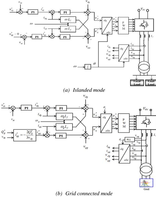
Figure 4. Converter control in islanded and grid connected modes
