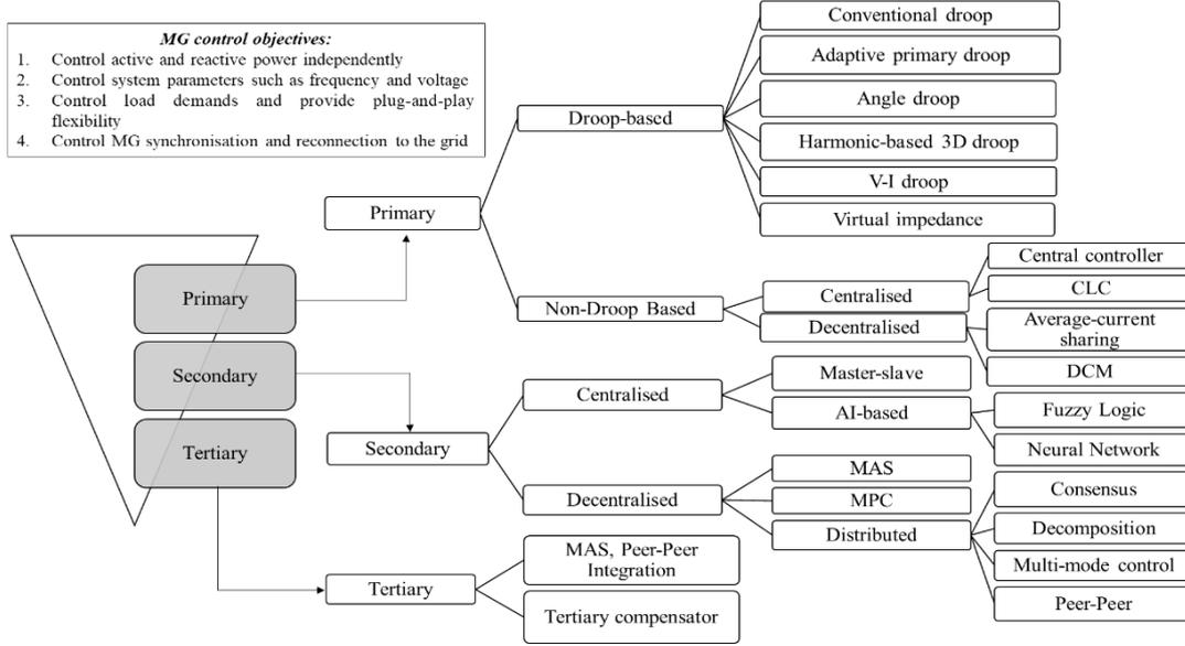
Figure 2. Hierarchical control in microgrids
