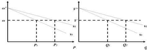
Figure 5. Conventional Droop characteristics in AC microgrids
