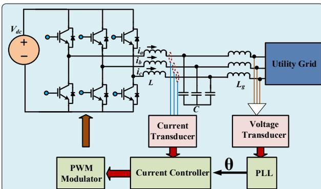
Fig. 1: Grid connected three phase inverter.
