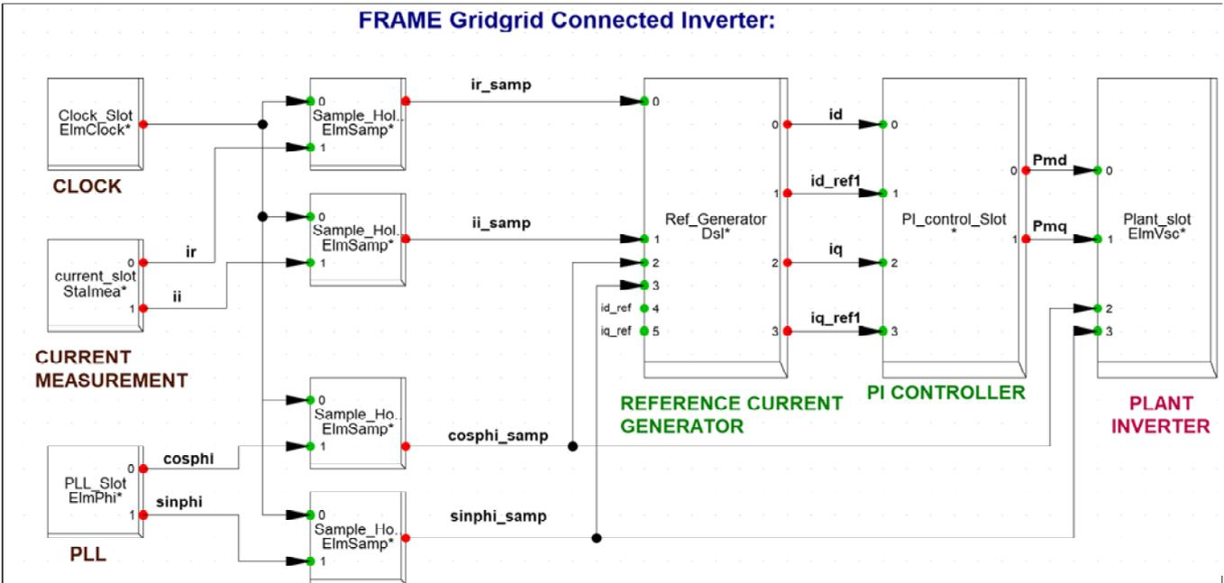
Fig. 6: DiGSILENT Composite Frame of the grid connected inverter with SRF current regulator.
