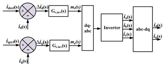
Fig. 3: Block diagram of inverter SRF PI controller.
