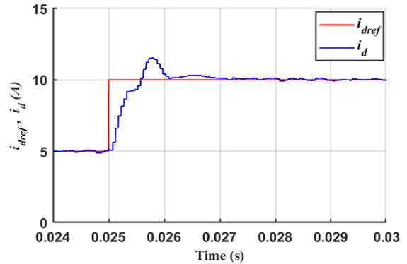
Fig. 10b: Transient performance: for step increase in input reference current (DIgSILENT results)
