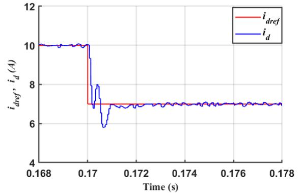
Fig. 14b: Transient performance: for step decrease in input reference current (DIgSILENT results)
