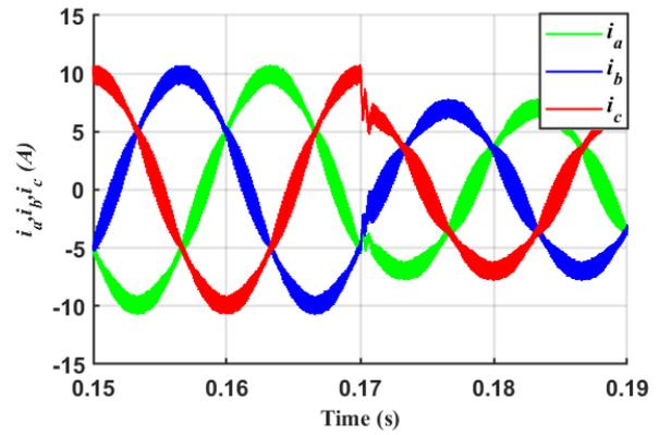
Fig. 13b: Inverter side inductor three phase currents for step decrease in input reference (DIgSILENT results)
