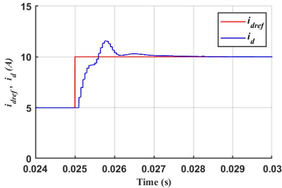
Fig. 10a: Transient performance: for step increase in input reference current (PSIM results)
