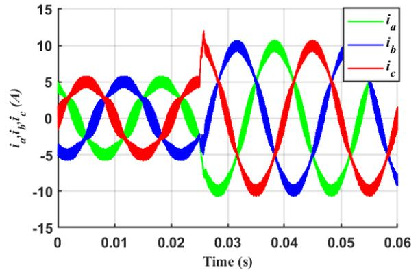
Fig. 9b: Inverter side inductor three phase currents for step increase in input reference (DIgSILENT results)
