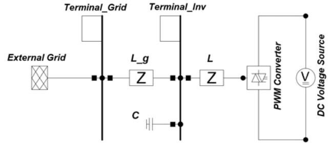
Fig. 5: Single Line Diagram (SLD) of grid connected three phase inverter.
