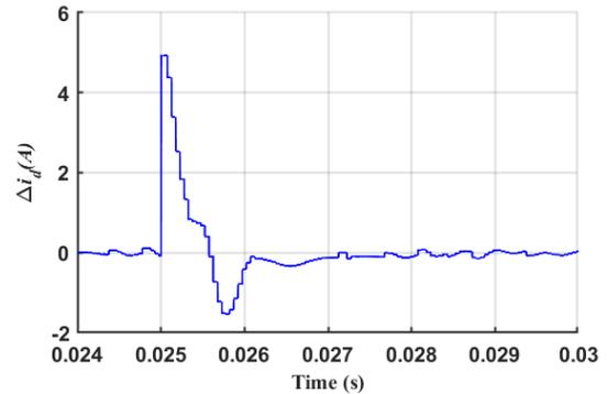
Fig. 11b: Steady state error: for step increase in input reference current (DIgSILENT results)
