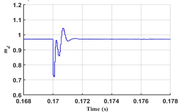
Fig. 16a: Modulating signal: for step decrease in input reference current (PSIM results)
