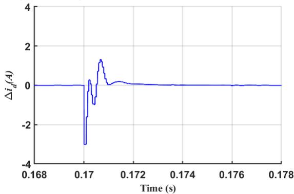
Fig. 15a: Steady state error: for step decrease in input reference current (PSIM results)
