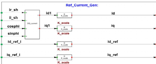
Fig. 7: DiGSILENT common model of reference current generation.
