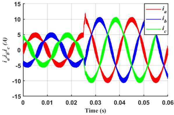
Fig. 9a: Inverter side inductor three phase currents for step increase in input reference (PSIM results)
