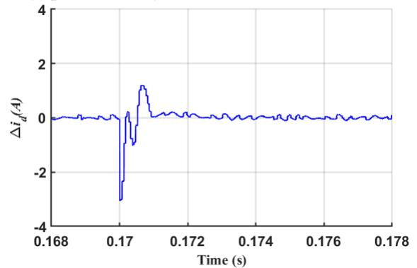
Fig. 15b: Steady state error: for step decrease in input reference current (DIgSILENT results)
