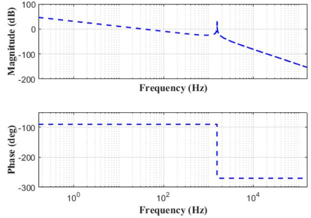
Fig. 2: Bode Plot of LCL filter attenuation admittance.
