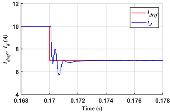
Fig. 14a: Transient performance: for step decrease in input reference current (PSIM results)
