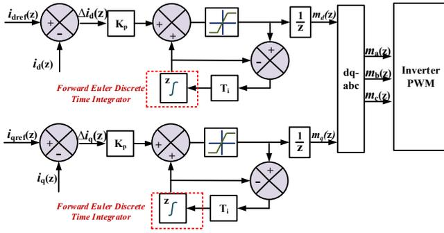
Fig. 4: Implementation of inverter SRF PI controller implementation in discrete time domain.
