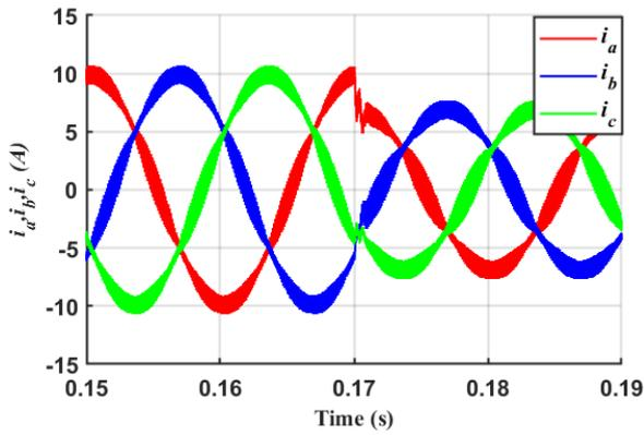
Fig. 13a: Inverter side inductor three phase currents for step decrease in input reference (PSIM results)
