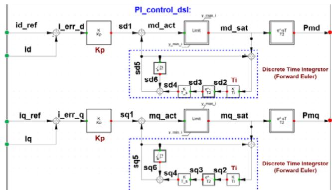
Fig. 8: DiGSILENT common model of PI SRF current regulator DSL.
