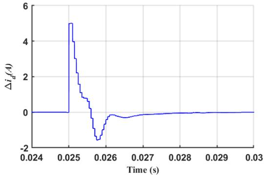
Fig. 11a: Steady state error: for step increase in input reference current (PSIM results)
