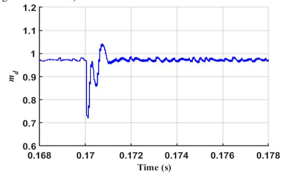
Fig. 16b: Modulating signal: for step decrease in input reference current (DIgSILENT results)
