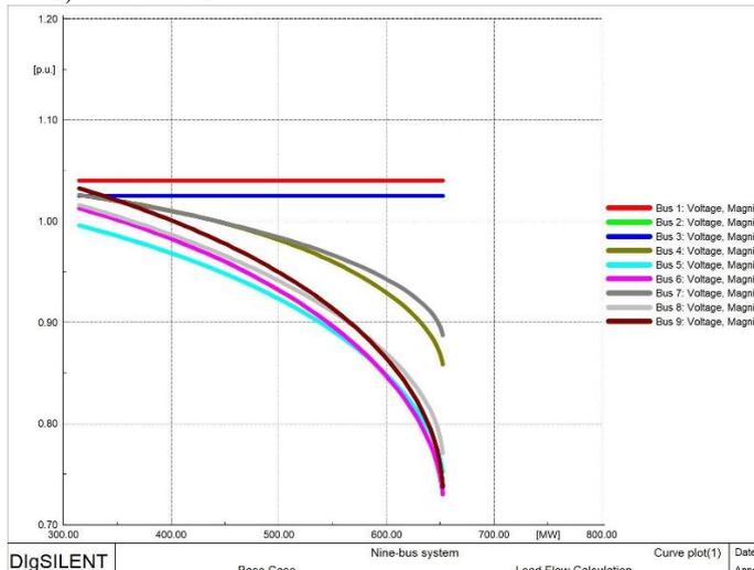
Figure 3: PV analysis of the system in scenario 2
