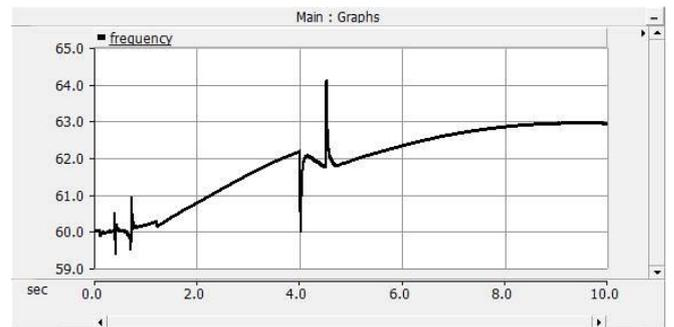
Figure 12: Frequency variation at bus 6 for a fault in scenario 3
