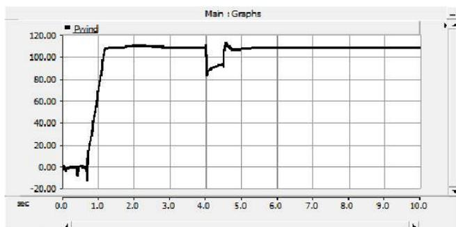
Figure 16; Active power output of the wind power plant for a fault in the system
