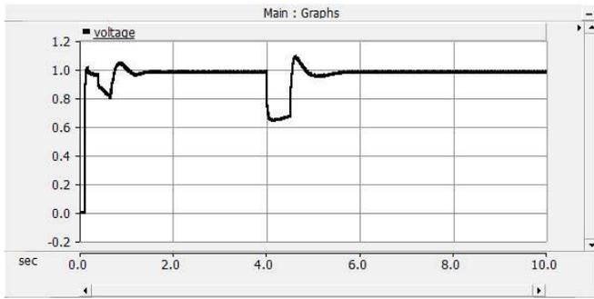
Figure 7: Voltage variation at bus 6 for a fault in scenario 2
