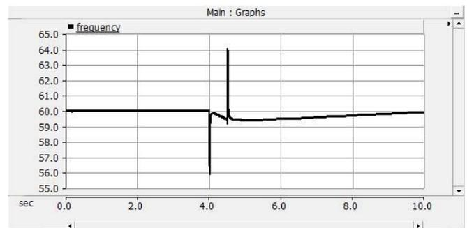
Figure 6: Frequency variation at bus 9 under a fault in scenario 1
