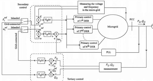
Figure 1: Hierarchical control of a microgrid [10]
