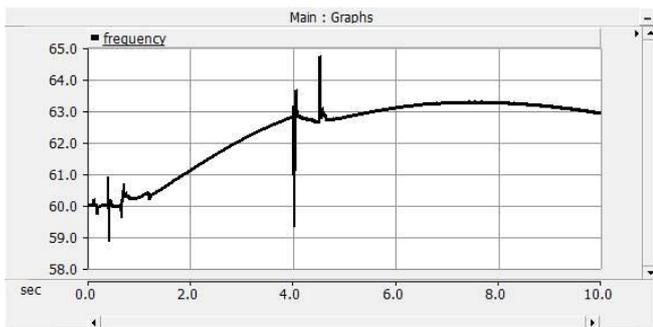
Figure 9: Frequency variation at bus 6 for a fault in scenario 2
