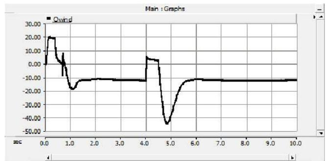
Figure 17; Reactive power output from wind power plant for a fault in the system
