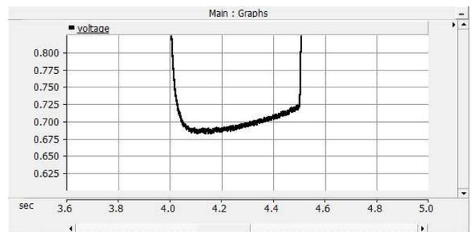
Figure 5: Voltage dip at bus 6 during a fault in scenario 1
