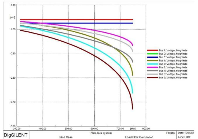
Figure 2: PV analysis of the system in scenario 1
