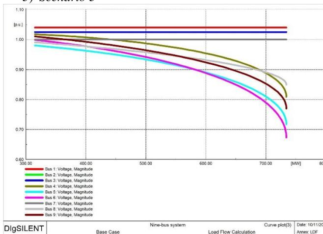
Figure 4: PV analysis of the system in scenario 3
