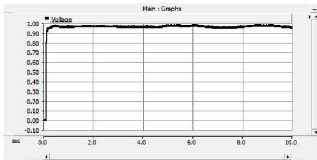
Figure 14: Voltage response at bus 6 for a gust of wind at 4 seconds
