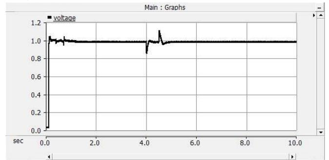
Figure 11: Voltage variation at bus 6 for a fault in scenario 3
