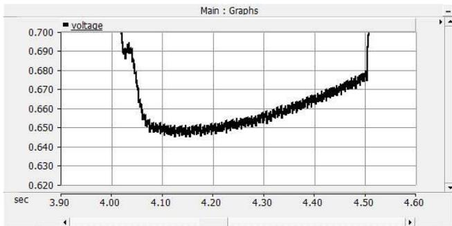
Figure 8: Voltage dip at bus 6 for a fault in scenario 2
