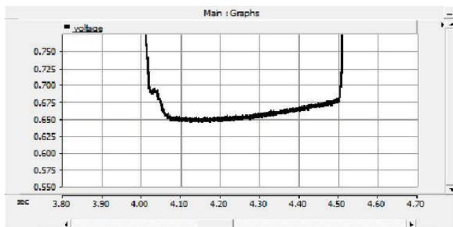
Figure 15; Voltage dip at wind power plant terminal voltage for a fault in the system
