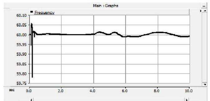
Figure 13: Frequency response at bus 6 for a gust of wind at 4 second
