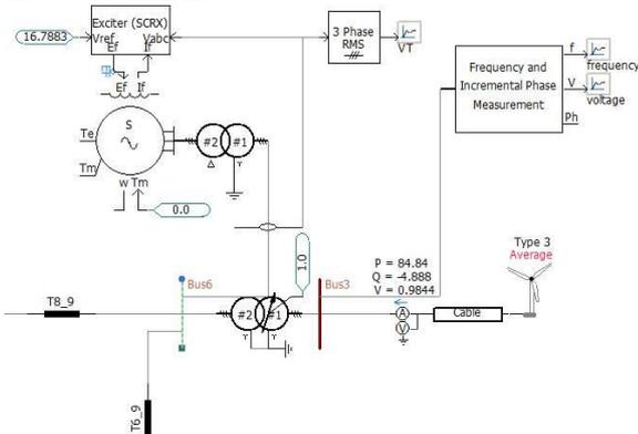
Figure 10: Synchronous condenser connected at bus 9(only a section of the system is shown)
