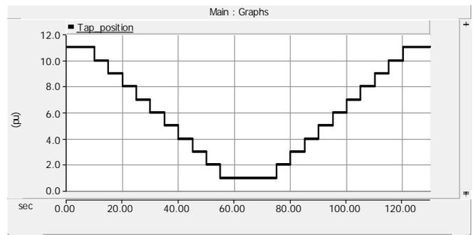
Figure 7: transformer tap position
