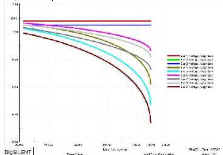
Figure 2: PV analysis of IEEE 9 bus system
