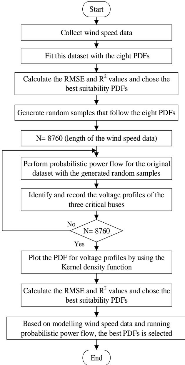
Fig. 1: The flowchart of probabilistic modelling of wind speed data.
