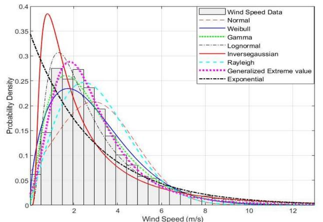
Fig. 3: The histogram of wind speed data fitted with the eight PDF.
