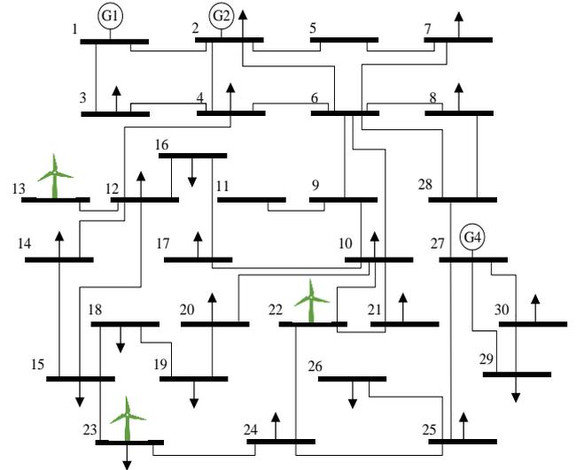
Fig. 2: The IEEE 30-bus test network.
