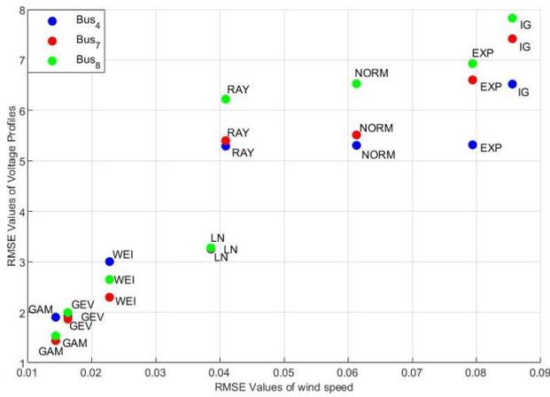
Fig. 9: Scatter plot of RMSE values of fitting wind speed data and voltage profiles analysis of the three critical busbars.
