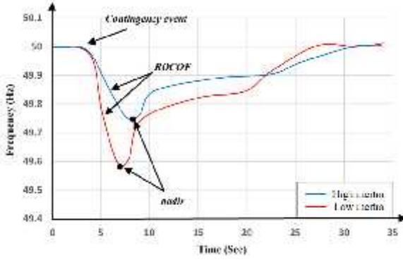
Fig. 1. Frequency nadir and ROCOF of high and low inertia power systems
