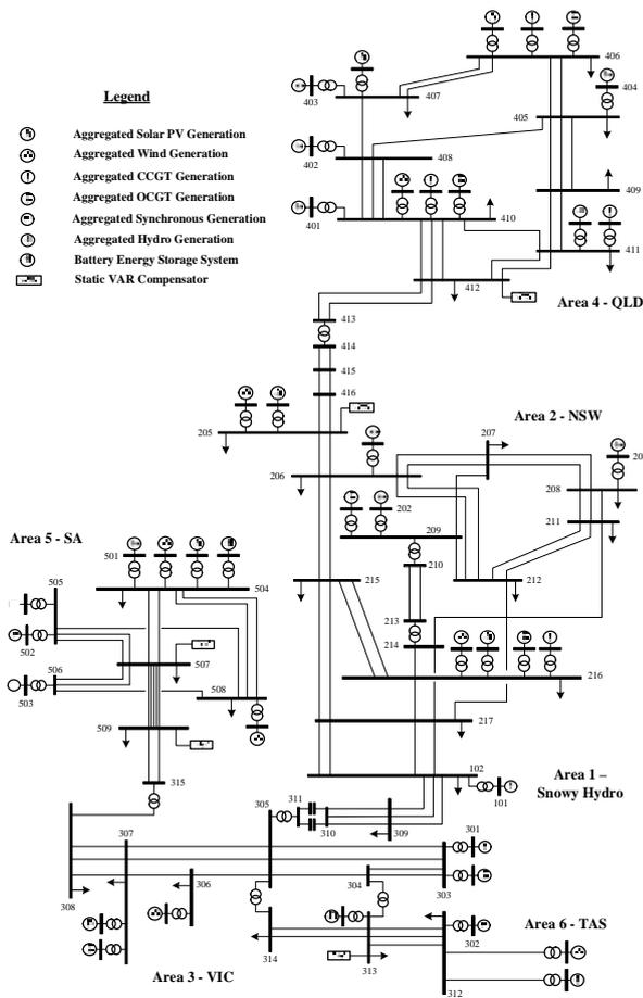
Fig. 6. Modified 14 generator South-Eastern Australian power system
