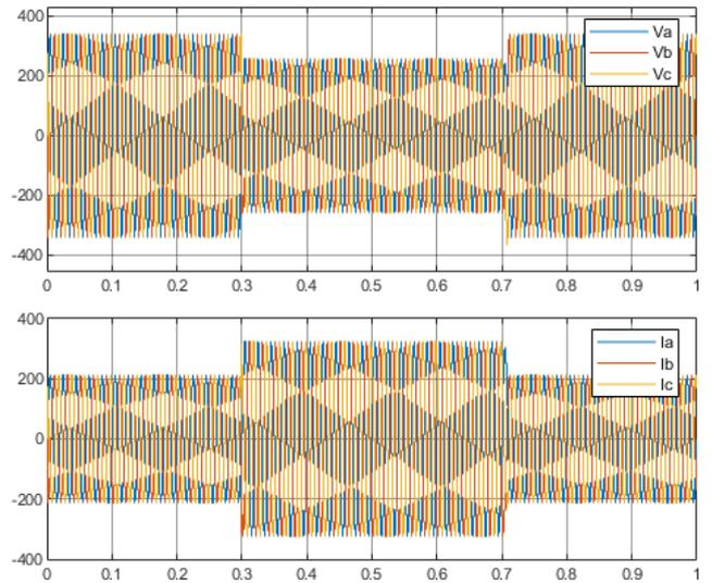
Fig. 10 Three phase voltages and currents of grid following converter with switching stage with a step change at 0.3s to 0.7s.
