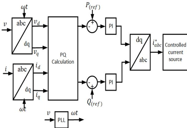
Fig. 5 Basic control structure for grid following converter without switching stage
