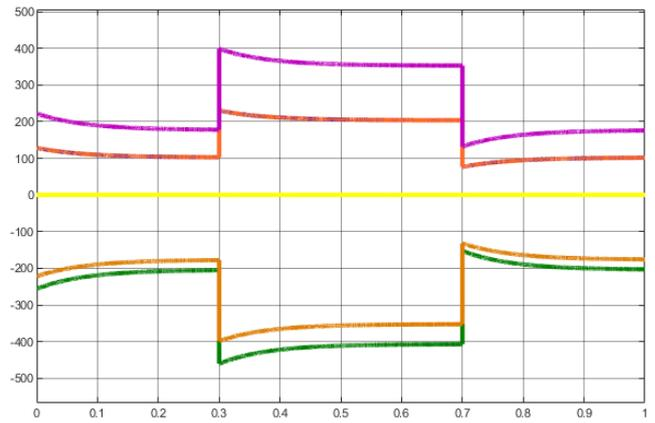
Fig. 9 Three phase voltages and currents of grid forming converter in phasor domain with a step change at 0.3s to 0.7s.
