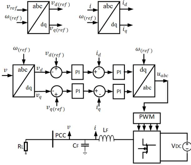
Fig.1 Basic control structure for grid forming converter including switching stage
