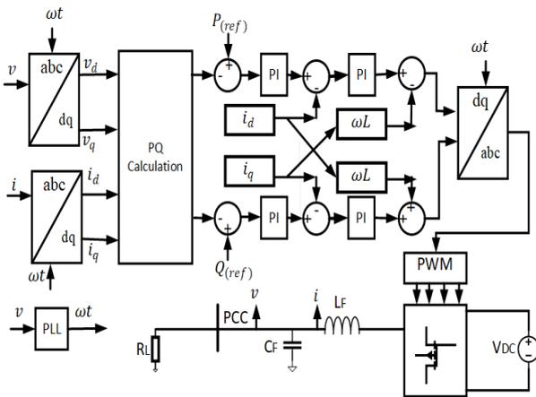
Fig. 4 Basic control structure for grid following converter with switching stage
