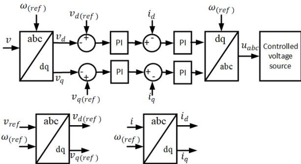
Fig. 2 Control structure for grid forming converter without the switching stage
