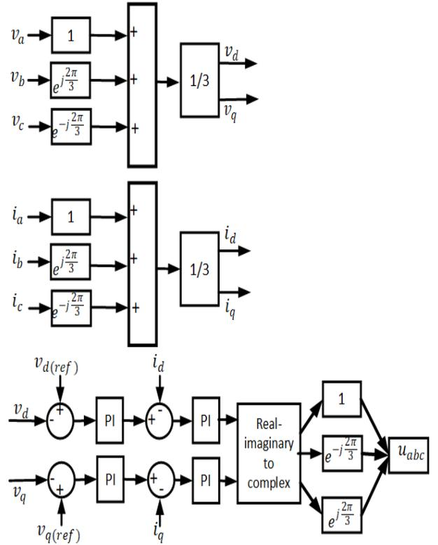
Fig. 3 Control structure for grid forming converter in phasor domain
