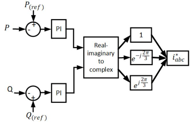
Fig. 6 Basic control structure for grid following converter in phasor domain
