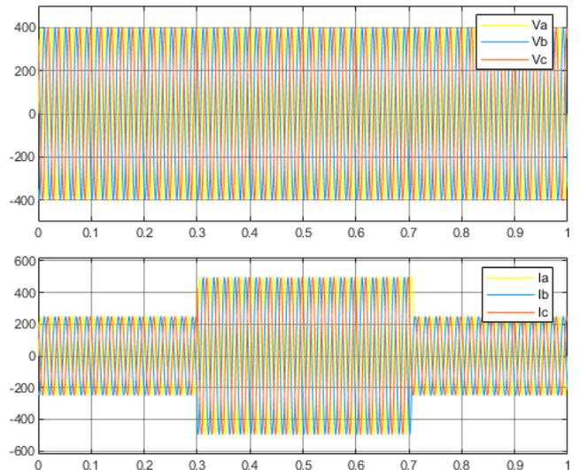
Fig. 11 Three phase voltages and currents of grid following converter with controlled current source with a step change at 0.3s to 0.7s.
