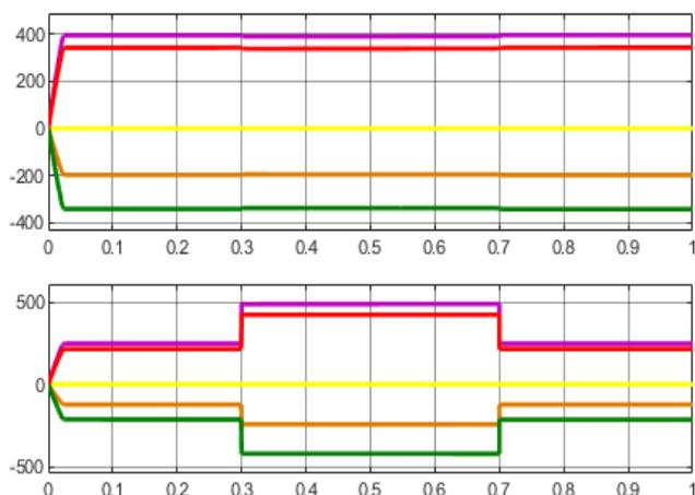
Fig. 12 Three phase voltages and currents of grid following converter in phasor domain with a step change at 0.3s to 0.7s.
