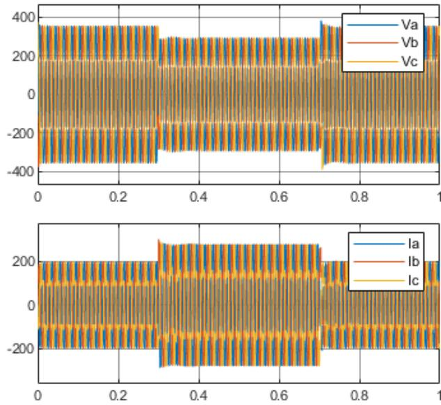
Fig. 7 Three phase voltages and currents of grid forming converter with switching stage with a step change at 0.3s to 0.7s.
