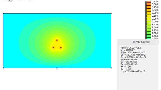
Fig. 4. Electric field of Delta configuration
