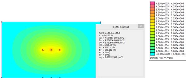
Fig. 2. Electrical field for Horizontal configuration
