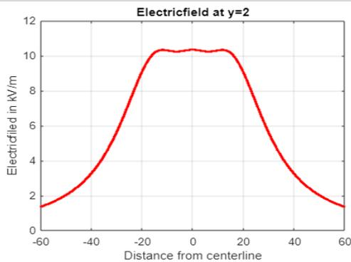
Fig. 6. Electric field at 2m above from ground
