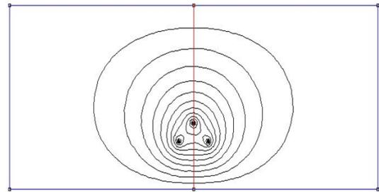
Fig. 5. Magnetic field for Delta configuration
