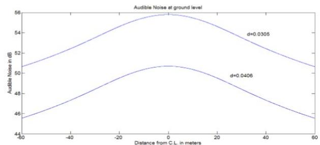
Fig. 12. comparison of AN for Two different sub conductor
