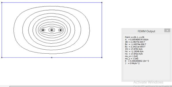
Fig. 3. Magnetic field for Horizontal configuration
