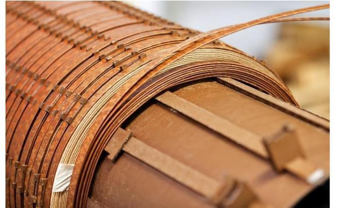
**Figure 6: An example of a winding with paper-wrapped conductor and pressboard structures – the impregnation of the insulating material's pours with insulating liquid is critical to ensuring the absence of voids and high effective dielectric strength.**
