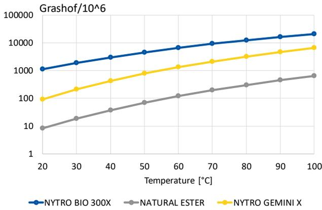
**Figure 3: The Grashof (Gr) number (divided by  $10^6$ ) calculated for the temperature range 20-100°C for NYTRO BIO 300X, NATURAL ESTER and GEMINI X. An increasing Grashof number indicates higher flow due to natural convection.**
