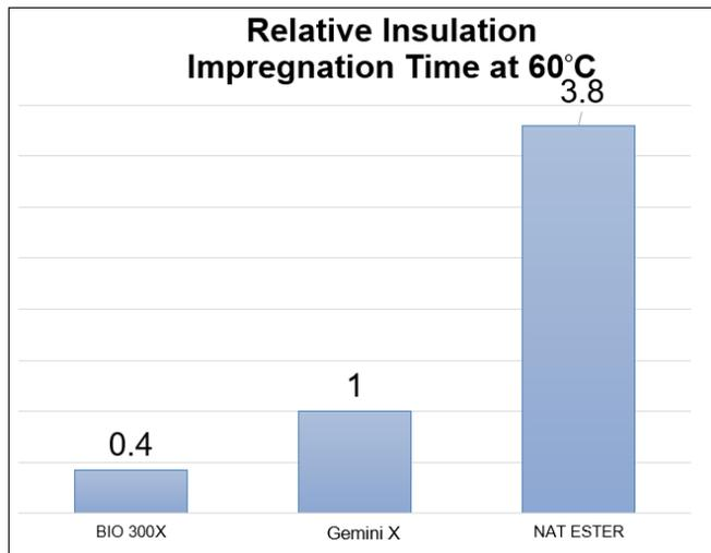
Figure 7 – An example of the approximate relative duration of insulation impregnation at 60°C. The natural ester will take 3.8 times longer than NYTRO Gemini X.
