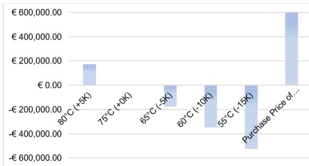
**Figure 5: Bar chart comparison of the change in total cost of losses from Table 1 based on changes on the average winding temperature. The potential savings in cost of losses from improved winding temperatures can be comparable to the purchase price of the transformer.**
