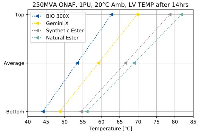
**Figure 2: Simulated LV winding temperature gradient for the different liquids (with same simulation parameters kept constant). The load is set at 1 PU, ONAF, ambient 20°C.**
