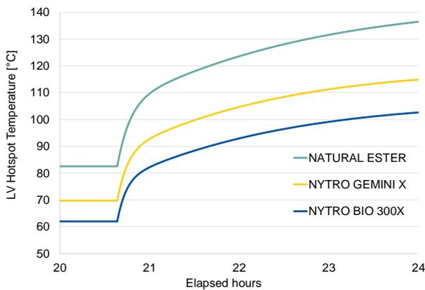
**Figure 1: Simulated LV winding hotspot – based on work and models developed in [1] – a 250 MVA ONAF (Oil Natural Air Forced) transformer with the same load and ambient conditions used for all liquid cases. The difference in viscosity primarily leads to the difference in cooling. The load is set at 1PU until a step change to 1.5PU for the remainder. Ambient 20°C.**
